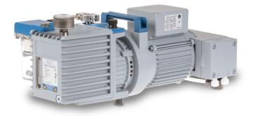
The RC 6 chemistry-HYBRID pump is the optimized corrosion resistant combination of a two-stage rotary vane pump and a chemistry diaphragm pump. The diaphragm pump continuously maintains the oil reservoir of the rotary vane pump under vacuum and prevents condensation in the oilsealed part under corresponding pressure and temperature conditions.
